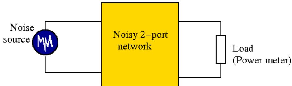
Figure 1: Noisy two-port showing input calibrated noise source and load (measuring device).
